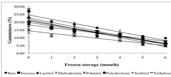
**Figure 8.** Changes in gumminess of surimi gel with different cryoprotectants during six months of frozen storage. Values shown are averages of triplicate analyses of duplicate surimi blocks. Data are shown as the mean  $\pm$  SD
